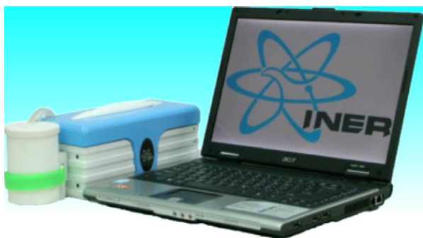
Fig. 13. A notebook PC powered by a portable DMFC system.
